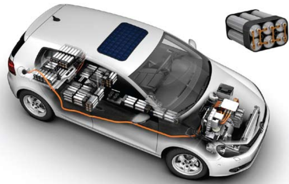
Battery modules are located beneath the rear floor, rear seat, and between the front seats.
